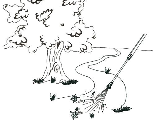
3. Rotating nozzle adjusts spray pattern from a narrow pattern to a fan pattern.
